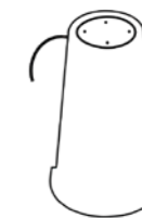
Water outlet pipe for excess water to flow out.
